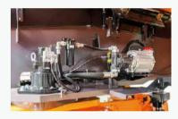
Permanent magnet motor drive variable piston pump, strong performance and low energy consumption.
